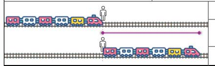
$$\frac{40 \text{ km}}{\text{hour}} = \frac{200 \text{ metre}}{\text{Time (seconds)}}$$
