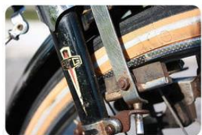
Friction between a bicycle brake pad and the rim of a wheel causes the wheel to stop turning.
